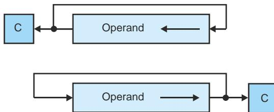
In a rotate operation, the bit shifted out is copied into the bit vacated at the other end (i.e., no bit is lost during a rotate). The bit shifted out is also copied into the carry bit
