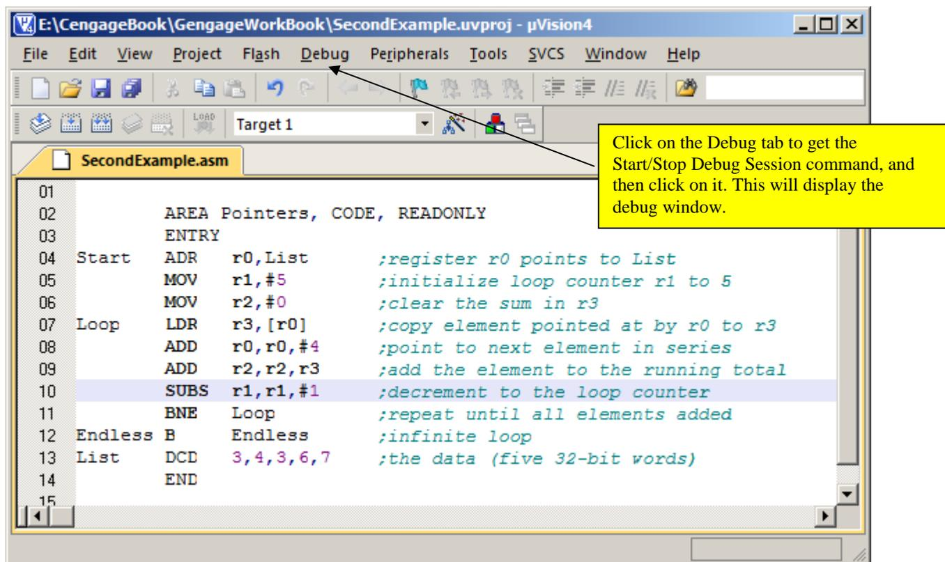
The next snapshot shows the result of entering the debug mode. For clarity, we have removed some of the windows that are not needed.
