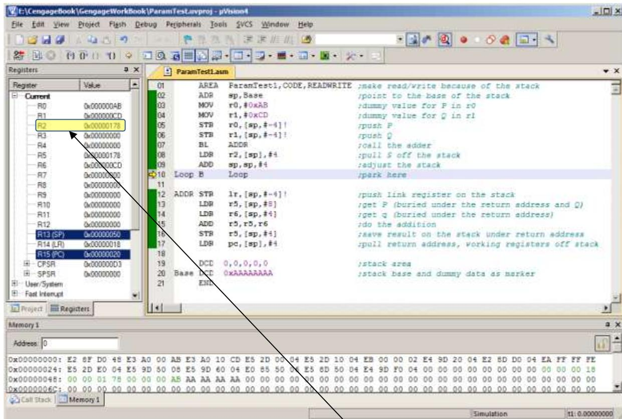
We have pulled the result off the stack and put it in r2.
