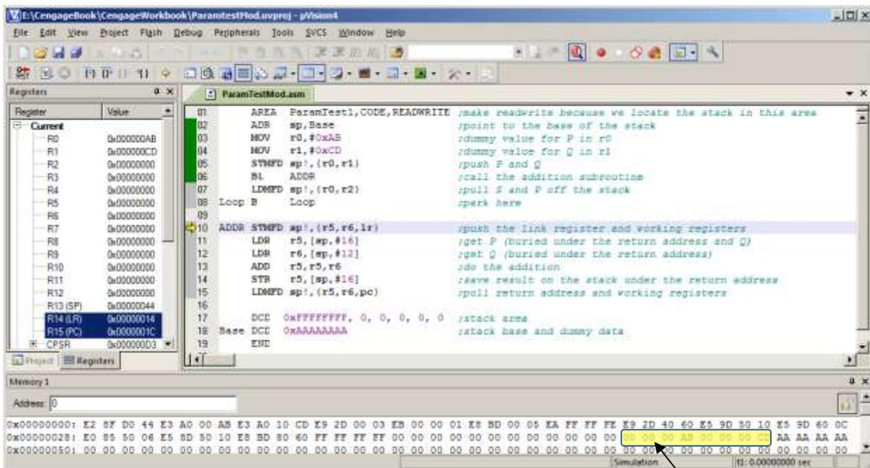
Here are parameters P and Q on the stack. Note that there are above 0xAAAAAAAA that we have used as a marker to show the base of the stack.
