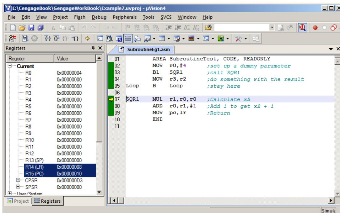
This subroutine mechanism has two flaws. First, because the multiply instruction can't use the same register for source and destination, we have to use  $r1$  to receive the result. This means that  $r1$  is used by the subroutine and any data in it will be overwritten. Second, this subroutine can't call another subroutine or be reused because the return address is in  $r13$ , the link register, and another subroutine call would overwrite it.
