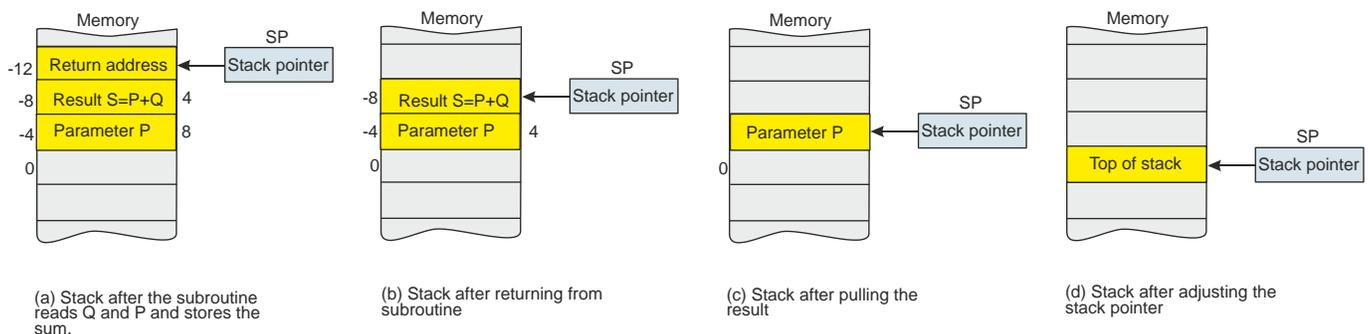
As you can see, the stack grows as parameters are pushed and the subroutine called. Then the stack declines as a return made and the two items on the stack removed. Now, let's look at this process in detail using an ARM processor.
