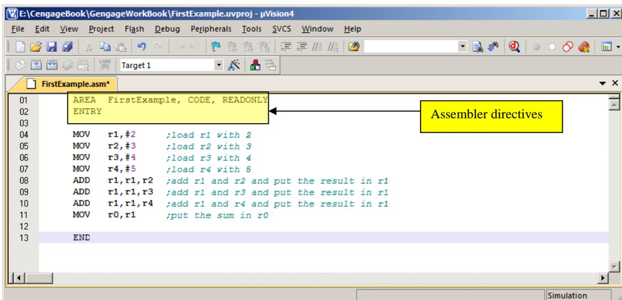
This program is simple. It loads register with numbers (literals), adds them together and then moves the result into register r0. Note that there are three lines that are not part of the assembly language. These are **assembler directives** that tell the assembler things it needs to know. The first assemble directive is
