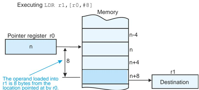
A typical application of pre-indexed addressing is in accessing a table. Consider a table in memory containing 12 entries corresponding to January to December. Register  $r0$  points at the start of the table (i.e., January). The following operations have the effect:
