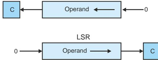
In a logical shift, a zero is shifted in and the bit shifted out is copied to the carry bit of the condition code register.
