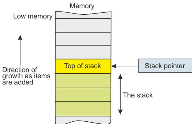
In this stack, the stack pointer points to the item at the top of the stack. This item is the last element pushed on the stack and will be the first item pulled off the stack (hence the term LIFO or *last-in first-out*).
