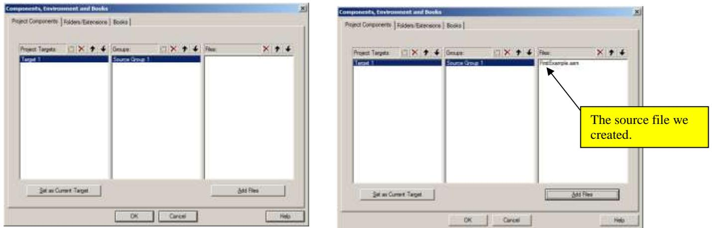
At this stage, we have a project, a processor, and a source file. Now we need to create the environment and assemble the code. Click on **Project** and then **Build target** from the drop-down window. The following image shows the screen after we have built the target.
