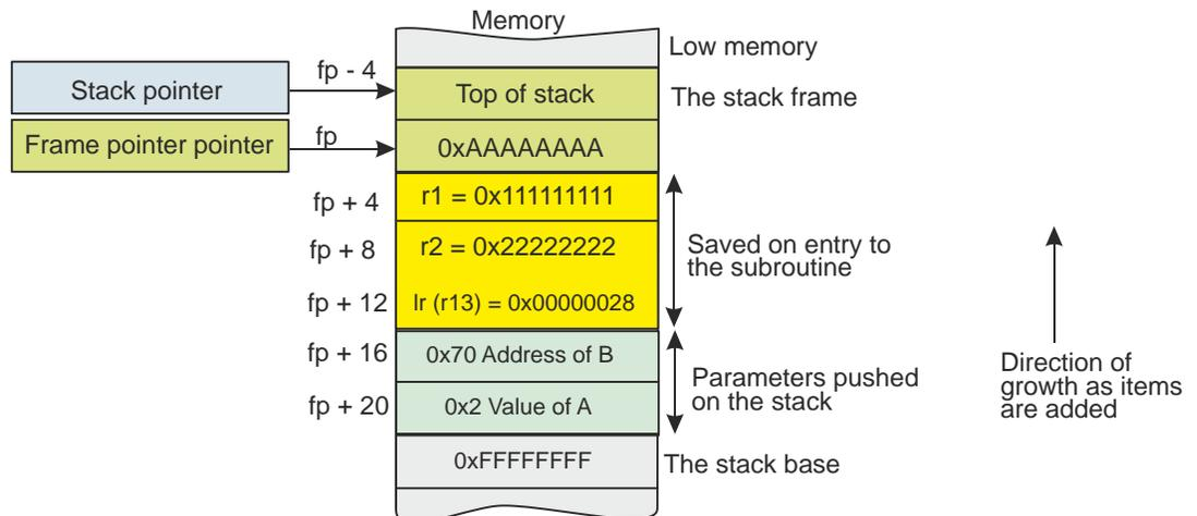
The following figure shows the memory map after squaring A and putting it in the stack frame.
