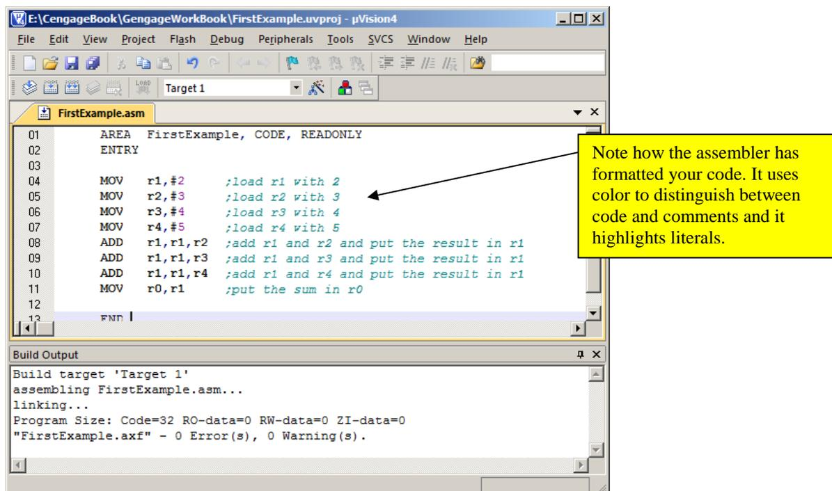
The **Build Output** window shows the status of the process. Here we are interested only in the magic words **0 Error(s)** that indicate all went well. Had there been any errors in the code, we would have been informed and would have had to edit the source file and then rebuild it. This cycle is repeated until there are no errors reported.
