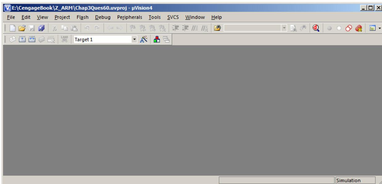
To start, select **Project** from the upper row of tabs and then **New  $\mu$ Vision Project** from the pull-down window. This brings up the **Create New Project** Window and you create a project name in the selected directory. I will use *FirstExample*. The development system automatically appends a file type to create **FirstExample.uvproj**.
