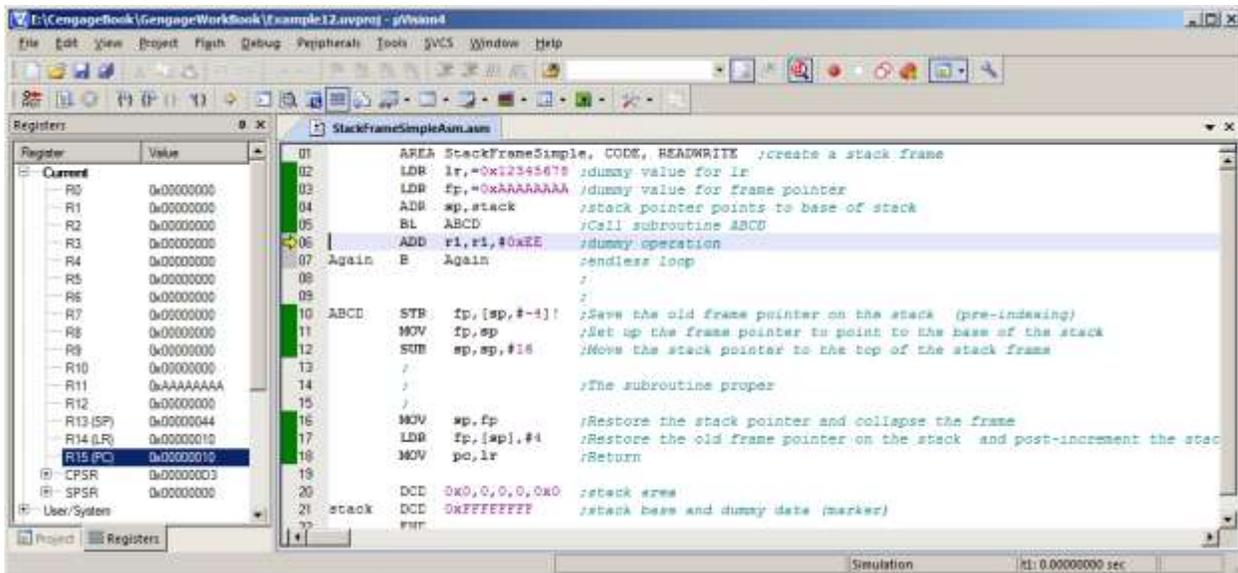
Up to now, we've demonstrated simple examples of stack frames. The next step is to provide a more realistic (albeit simple) example. This example will demonstrate various aspects of machine-level programming; for example, the use of registers (global and local), the use of temporary storage (stack frames), and parameter passing.
