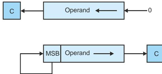
In an arithmetic shift, the number is either multiplied by 2 (ASL) or divided by 2 (ASR). The sign of a two's complement number is preserved.
