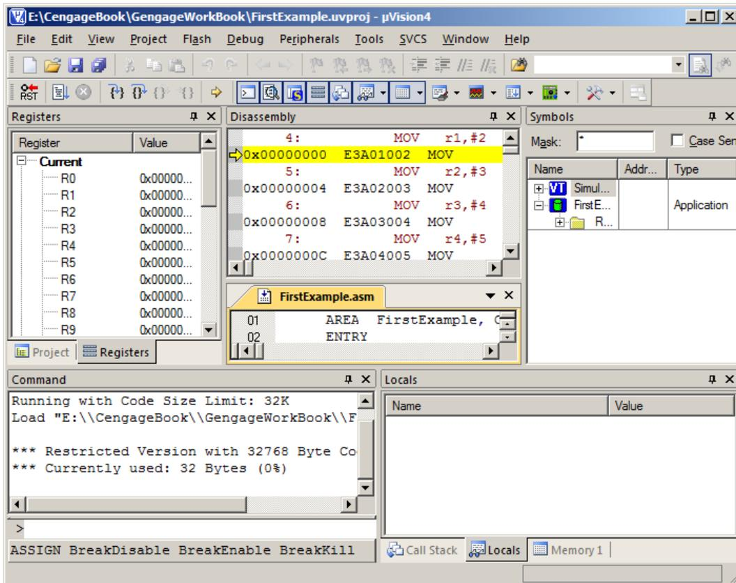
We don't need all this. Using normal Windows features we can resize and remove windows not of immediate importance to get the following image. We now have three windows. On the left there is a window, **Registers**, showing the contents of registers. All values are in hexadecimal. The other items (which have expansion boxes) are not of interest at the moment; these describe the status of the processor and the value of carry and overflow bits etc.
