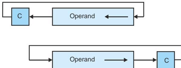
A circular shift operation treats the data being shifted as a ring with the most-significant bit adjacent to the least-significant bit. Circular shifts result in the most-significant bit being shifted into the least-significant bit position (left shift), or vice versa for a right shift. No data is lost during a circular shift. Consider the following examples.
