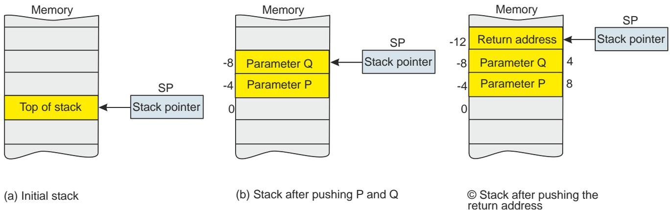
The next figure demonstrates the behavior of the stack during the subroutine execution.
