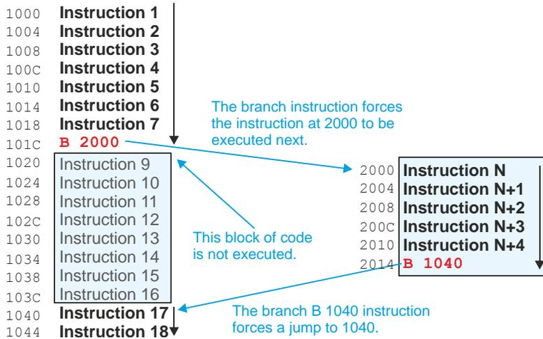
We have already used a simple unconditional branch in ARM programs when we wrote `Here B Here` when we wanted to force the computer into an infinite loop at the end of a program.
